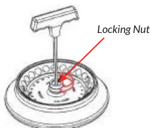
Load the Rotor Onto the Shaft
